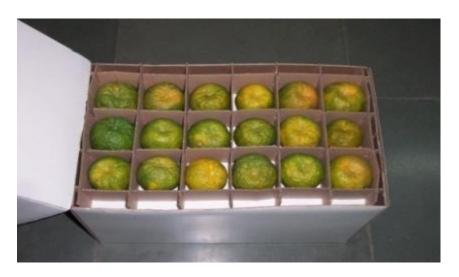
PHOTOGRAPH – 49 TELESCOPIC STYLE (0320) WITH SLOTTED PARTITIONS
